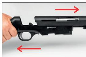
4. Pull the bolt handle half of the way back. Unscrew the bolt handle screw with special allen and remove it from the bolt.
