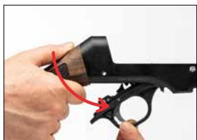
**8. For Wooden Buttstock;** To disassembly the wooden buttstock, unscrew the recoil pad screw and pull the recoil pad backwards. After removing the recoil pad, unscrew buttstock assembly screw with using special tool (5mm Allen Wrench Set) for it and separate them.
