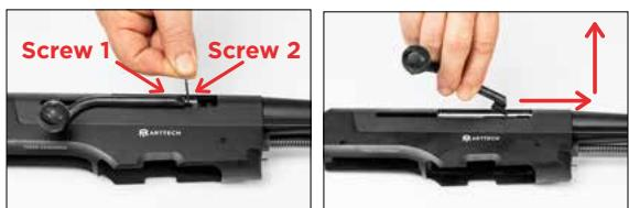
5. To remove the bolt carrier, separate the slide from the slide levers with a straight screwdriver After that hold the bolt carrier and pull it all the way back.
