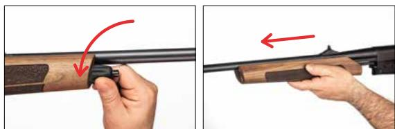
3. Hold the barrel group with one hand and hold the lower receiver with your other hand, at the same time. Remove the upper side from the lower receiver by pulling it forward..
