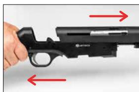
4. Pull the bolt handle half of the way back. Unscrew the bolt handle screws with special allen and remove them from the bolt.
