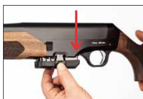
2. Unscrew the forend nut and push the forend forward while holding the receiver.
