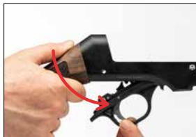
**8. For Wooden Buttstock:** To disassembly the wood buttstock, unscrew the recoil pad screw and pull the recoil pad backwards. After removing the recoil pad, unscrew buttstock assembly screw with using special tool (5mm Allen Wrench Set) for it and separate them.
