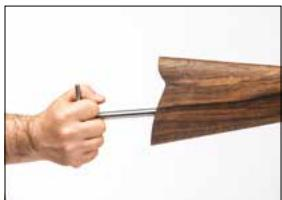
**For Synthetic Buttstock;** To diassembly the buttstock, push the recoil pad plunger pin and pull the recoil pad backwards. After removing the recoil pad, unscrew buttstock assembly screw with using special tool (5mm Allen Wrench Set) for it and separate them.
