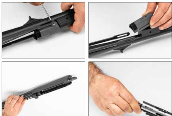
6. To remove the barrel from the upper receiver, unscrew the barrel assembly screw with 12mm wrench and separate them.
